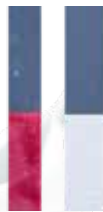
Working of the sucrose detection strip. The development of pink colour indicates presence of sucrose in milk
