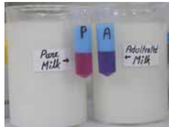
The blue colour in lower layer indicates milk sample adulterated with detergent whereas purple colour in lower indicate pure milk sample
