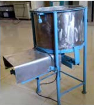
Developed whey dewatering mechanism for Channa unit
