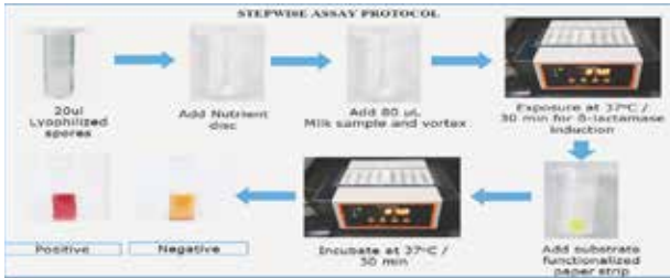
Step wise protocol of working of assay for Detection of \beta -Lactam Group in Milk
