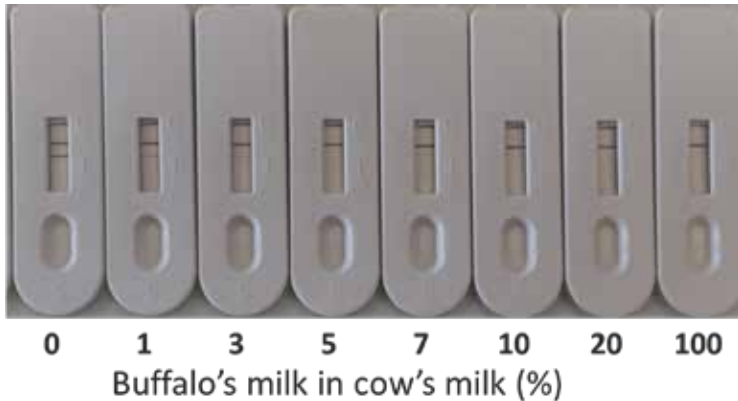
Lateral flow assay strips displaying results for rapid detection of presence of buffalo milk in cow milk
