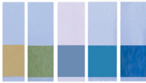
Original Strip Pure Milk Milk Adulterated with Sodium Hydroxide at Various Levels
