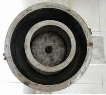
Whey dewatering mechanism for channa – top view and internal structure
