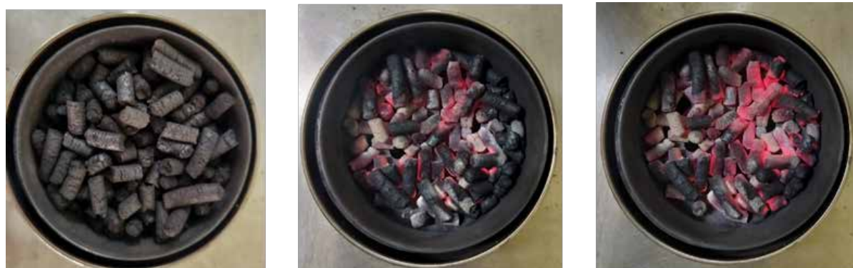
Torrefied cattle dung pellets for generation of bioenergy
